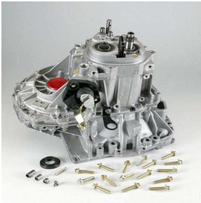
Gearbox. Including the differential case
